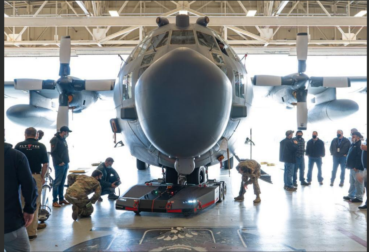
TF6 MilSpec testing on a C-130 at Hurlburt Field
